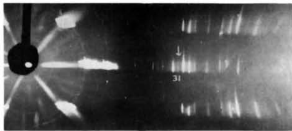
Fig. 1. X-ray a axis 15^\circ oscillation photograph of polytype 12R ; the angle between the incident beam and c varies between 25 and 40^\circ ; \text{Cu } K\alpha radiation, camera radius 30 mm. The arrow indicates the l value of a 01.l reflexion.
